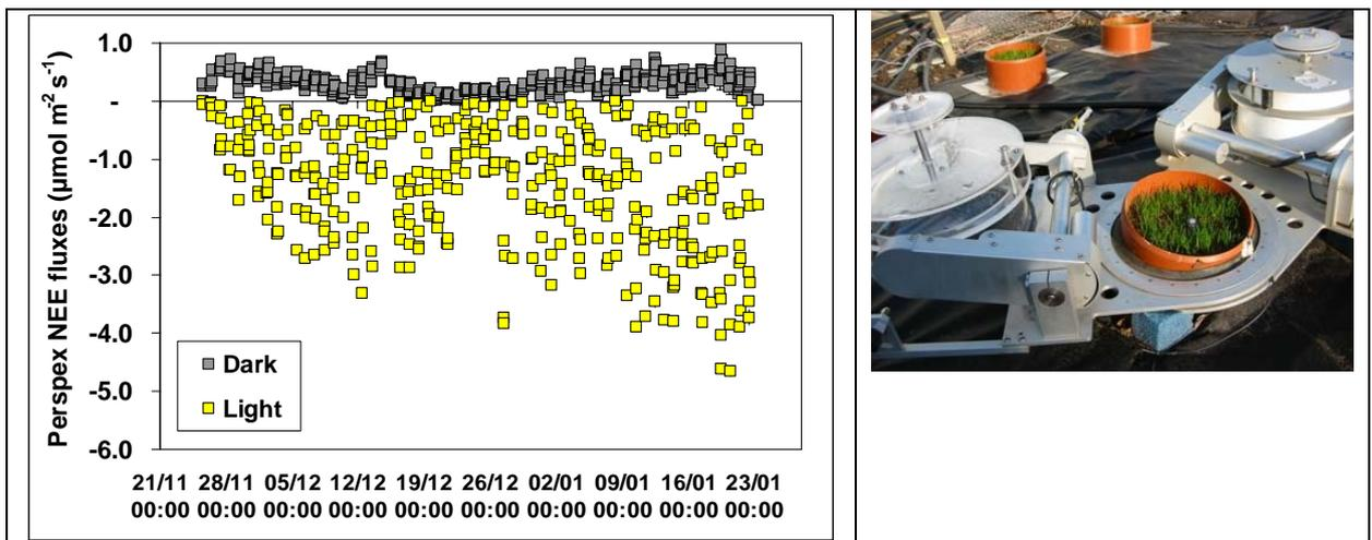
Figure 18-7: Data from the York multiplexed and continuous monitoring soil level NEE chamber system. Shown are hourly CO<sub>2</sub> fluxes from dark respiration (grey) and clear NEE perspex (yellow) chambers (see picture). Note the high net CO<sub>2</sub> uptake during the day (negative NEE values) starting immediately after seed germination (around 20th November 2006).
