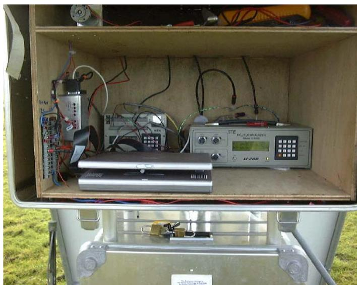
Figure 2: Interior of the flux monitoring station showing Licor IRGA, datalogger and eddy covariance computer
